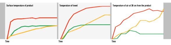
Tests performed at an ambient temperature of  $22^{\circ}\text{C}$  + $-2^{\circ}\text{C}$  compare the HELISEA 110 towel-warmer heater (RED LINE) with towel-warmer radiators featuring an equivalent electrical input and size but based on traditional heating technologies: products with internal fluid circulation (YELLOW LINE); products with a standard heating element (GREEN LINE).
